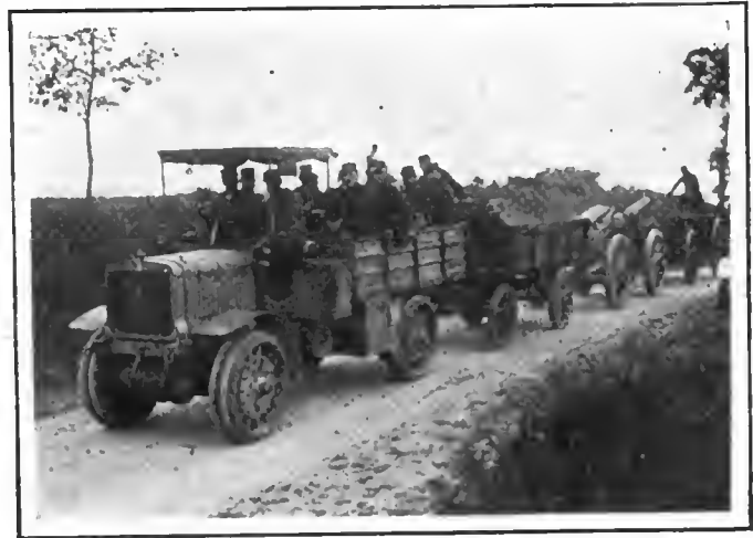
Panhard tractor hauling 155 millimeter siege guns and ammunition wagons
